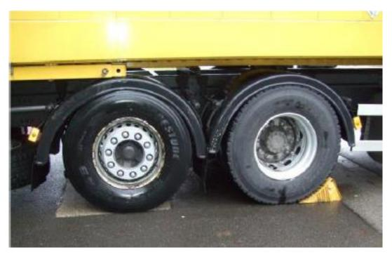
On every loading procedure, the driver must ensure that the HGV is secured so that it does not roll back. In order to do so, the driver must apply the parking brake and use wheel chocks.
