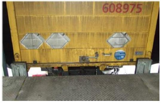
Manoeuvre vehicle flush with the raised ramp pad.
